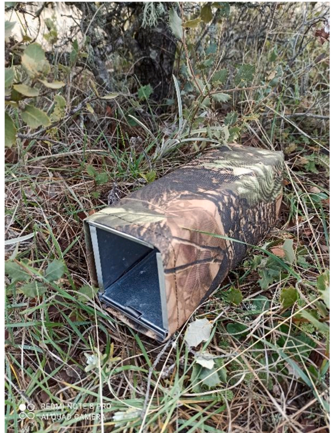
Fig. 1. Camouflage PVC cover designed for medium-sized Sherman traps (design by Paco Bustamante).
